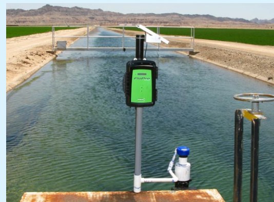
Figure 2: The Series3 MACE FloPro unit installed on Quail Mesa Ranch. An ultrasonic depth sensor (EchoSpan®) is mounted over the crest of the weir.
